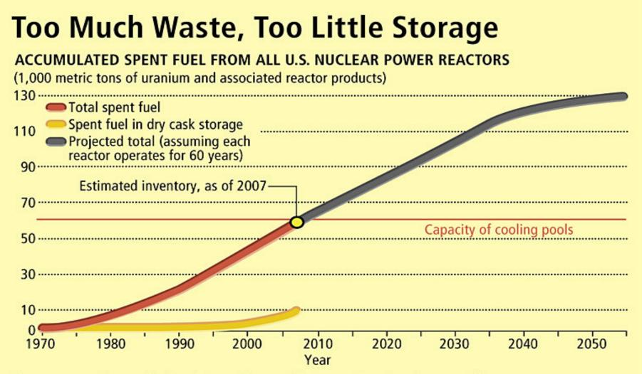
The amount of spent fuel will rise substantially in coming decades even if no new reactors are built. Managers at nuclear power plants increasingly are forced to transfer the oldest spent fuel in their cooling pools to dry casks situated close by. Not surprisingly, the industry is pressuring the U.S. government to help find a solution to the problem.
